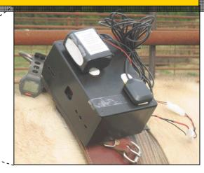
Ambulatory data acquisition with real-time transmission to a base station
